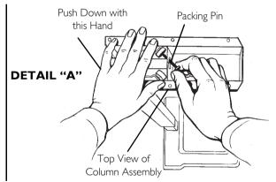
**FIGURE I** Assembling the Overbed Table
